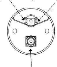
Tubing attachment 1/8-27 NPT threads
